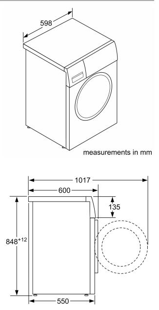
measurements in mm
