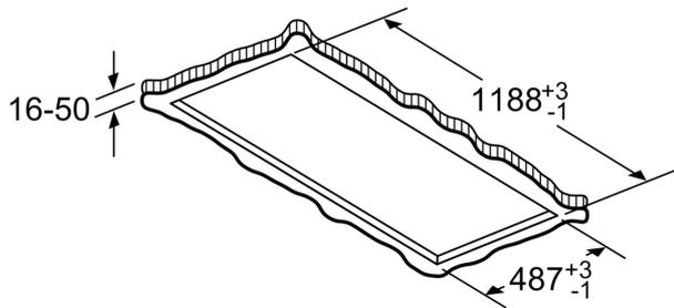
Never fit directly onto plasterboard or similar lightweight construction materials of the suspended ceiling. A suitable substructure is required that is securely fixed to the concrete ceiling.
