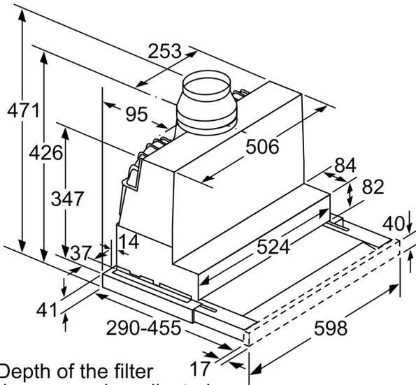
Depth of the filter drawer can be adjusted by up to 29 mm
