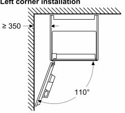
If using the 92° hinge limiter, the min. distance to the wall is only 100 mm  $\,$
