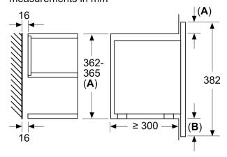
A: Overhang at top: Recess 362: 6 mm Recess 365: 3 mm
